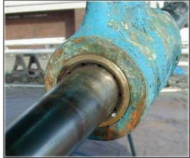
The above photo shows how cleaning the strut face thoroughly will clearly reveal the bearing outer shell for most accurate measuring.
