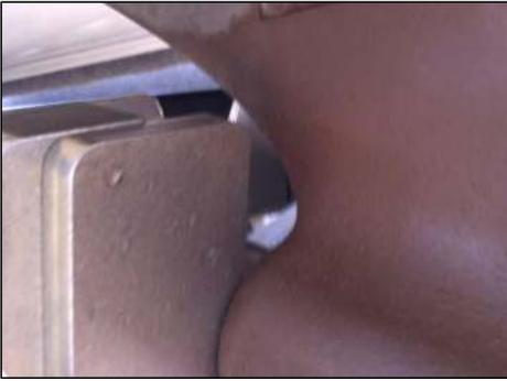
This close up photo shows a strut with the horseshoe inverted and facing upward. This method provides clearance so the horseshoe does not contact the leading edge of the strut. Steep strut angle is common on v-drives and certain small inboard vessels.
