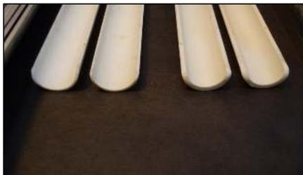
These special non-metallic spacers are provided for 3/4" and 7/8" shafts. They space the 1-1/4" o.d. x 1" i.d. collets away from the shaft to match up the two smallest shafts.
