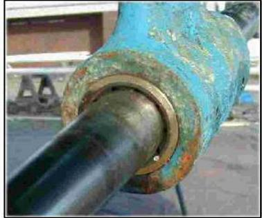
The above photo shows how cleaning the strut face thoroughly will clearly reveal the bearing outer shell for the most accurate measuring.
